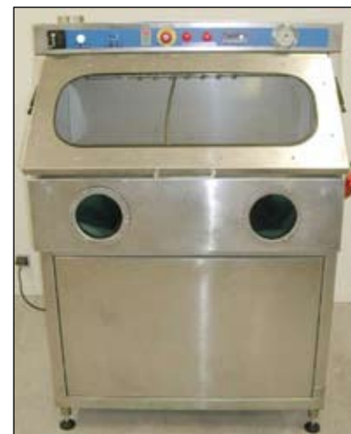
Figure 5 – NP15 cleaning machine (prototype developed by m.b.tech according to Matra Électronique's specifications)
